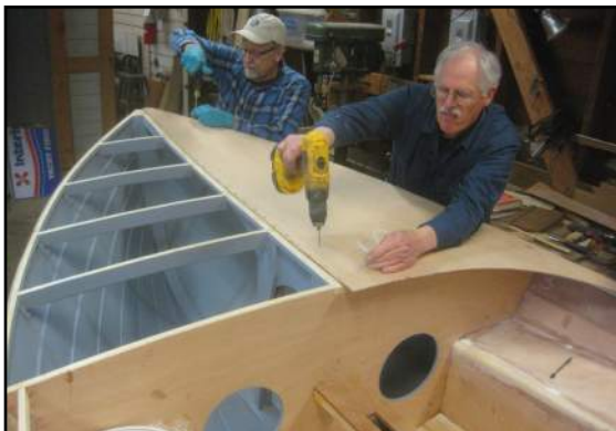
Rick Meyer and Bob Zimmerle install the Gannet foredeck in early March.
